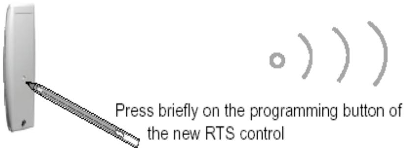
Hold down program button behind the remote control for 7 seconds until the motor moves upward-downward for two times. The motor moves upward and downward and repeats this action after 3 seconds and then memory is cleared. By doing so, motor memory is reset to factory setting.
